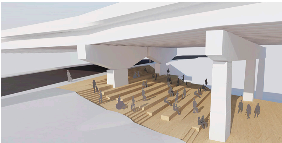
At Strachan Avenue a timber staircase with integrated ramps for barrier-free access forms an iconic entrance to the site from the street. It will also serve as an informal bleacher system to the stage below. (Image courtesy of PUBLIC WORK)
