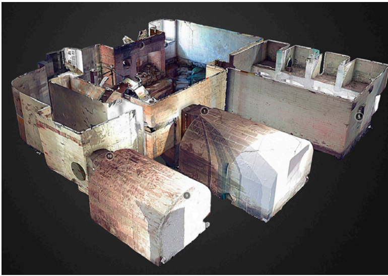
Three-dimensional model from lidar (light/laser detection and ranging) data showing the Officers' Mess Establishment cellar, including the two money vaults (foreground), with creative projection of vault ceiling photographic imagery onto the external structure of the vaults, which are inaccessible to the lidar scanner. The room's configuration is somewhat different from the way it was in the 19th century. The recording, using a Faro Focus 3D scanner, and subsequent modelling, was completed by volunteer Stephen Vickers (Carleton University) working with Ellis Don and ASI Heritage, during excavation of the schooner southeast of Fort York (see "Mystery ship arrives at Fort York" F&D, July 2015). After the excavation, Stephen volunteered to work with City of Toronto Museums staff to try recording the cellar. The successful scanning of the cellar prepared the way for the full 3D recording of Fort York by CyArk (see "The electronic capture of Fort York" F&D, December 2017).
